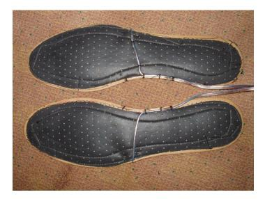
Step 2: Carbon tape covered by a thin cloth.
