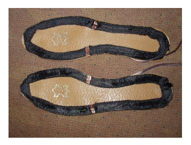
Step 1: It's powered by 1x18650 for each one. 3,7V x 1,3A almost 5W.
